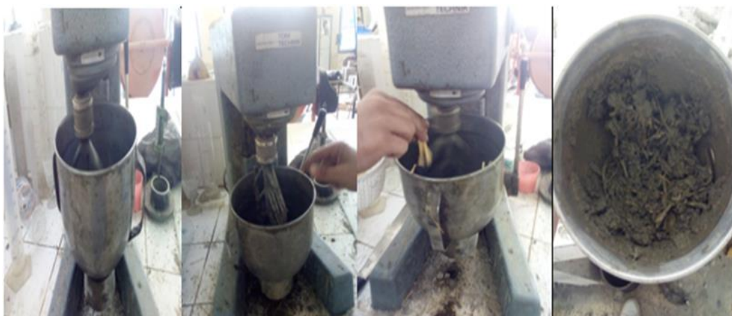
Figure III.8 : Elaboration des mortiers.
