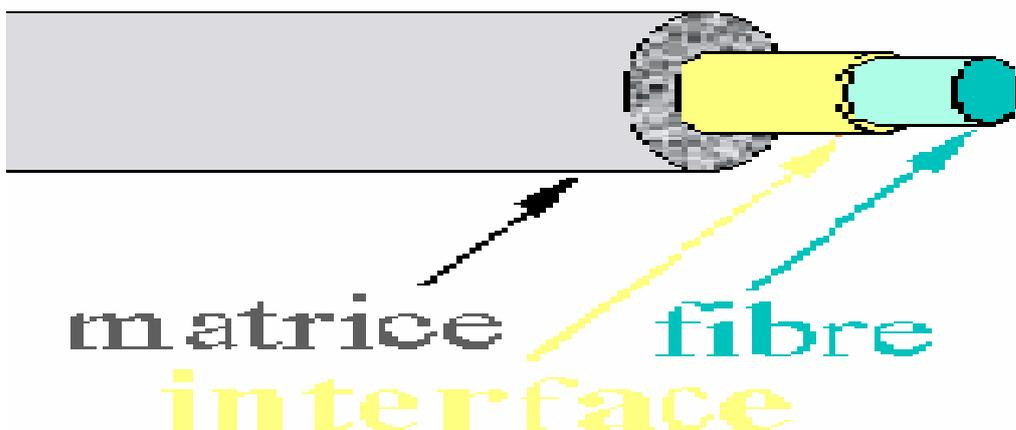
Figure II.1 : interface fibre matrice.
