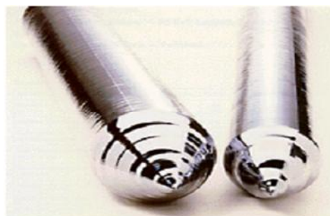
Figure I.8: Lingots de silicium monocristallin [20]
