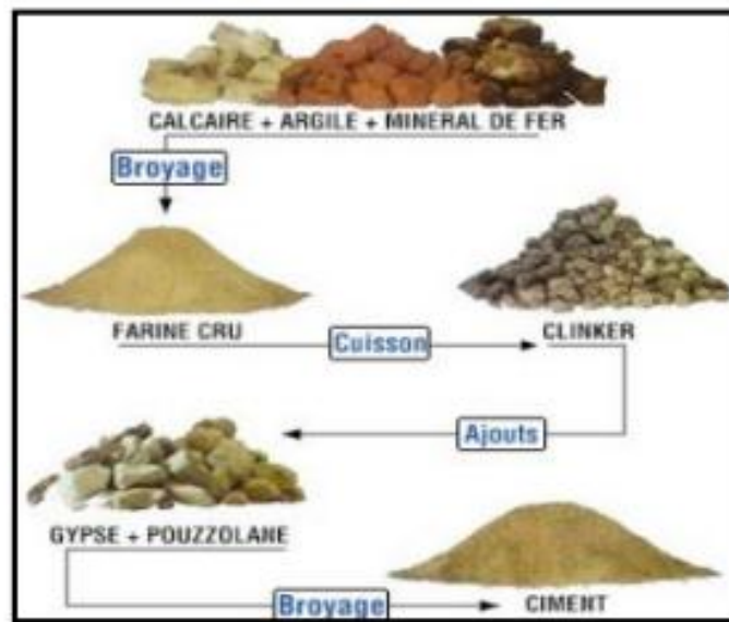
Figure III.5. Processus de fabrication de ciment
