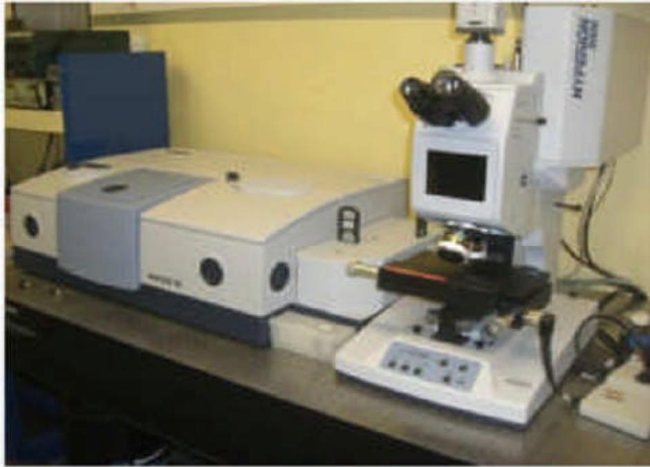
Figure II.12. Microscope FTIR.
