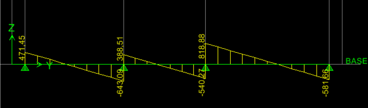
Figure VII.7.f effort tranchant a l'ELU (sens transversal)
