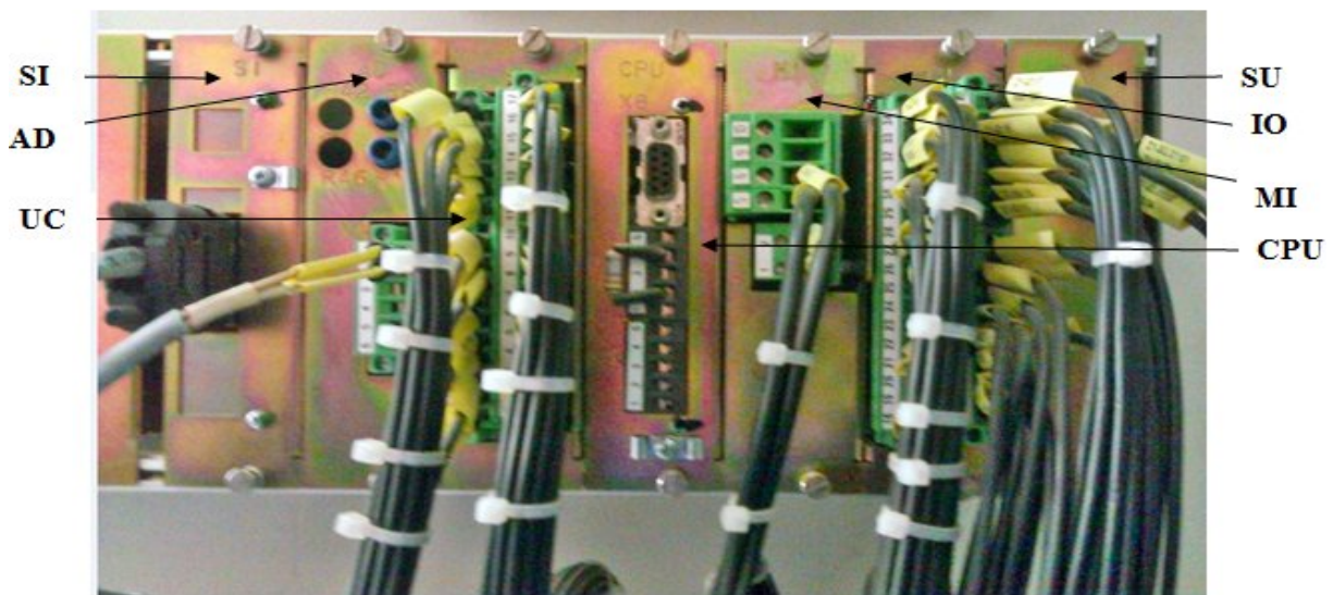
Figure IV.5 : Raccordement du TAPCON 240
