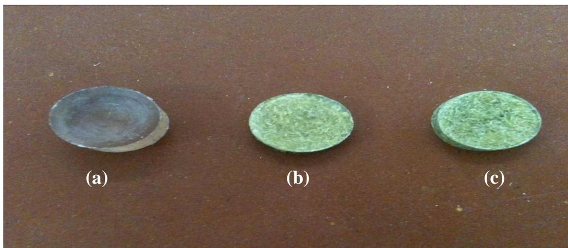
Figure III.4 : Les composites : (a) PVC pur, (b) PVC20, (c) PVC 20T.
