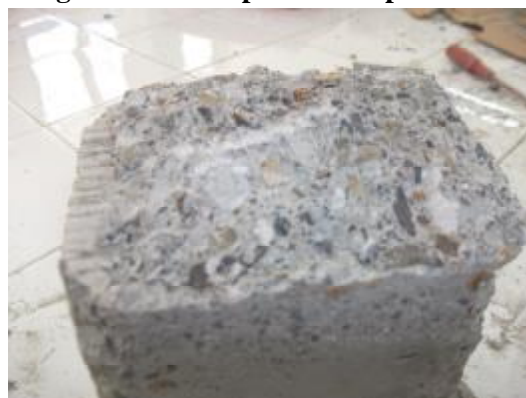
Figure II.24 : Surface de rupture
