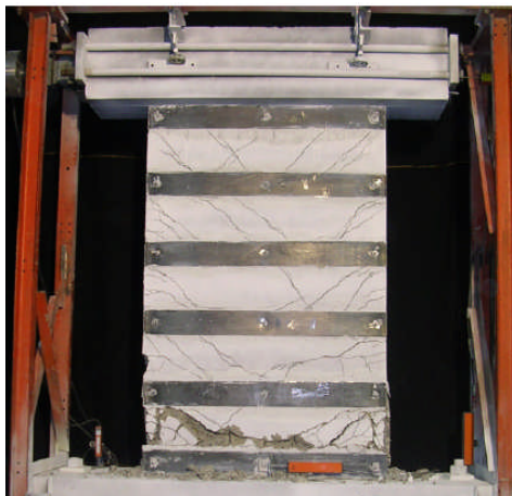
Figure III.18: Fissuration du spécimen 3.
