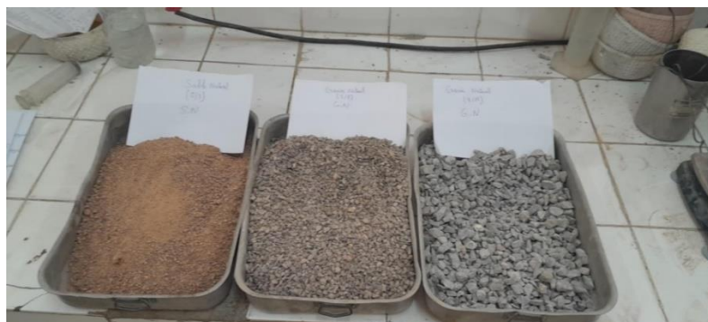
Figure II.4 : sable (0/3) et gravier naturel (3/8) (8/15) sec.
