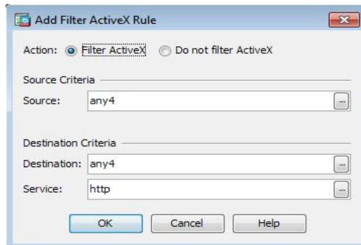
Figure 3.20 : Activation filtre ActiveX
