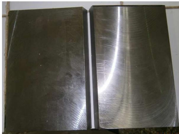
**Figure 4.2:** Deux plaquettes acier A60 /acier E36
