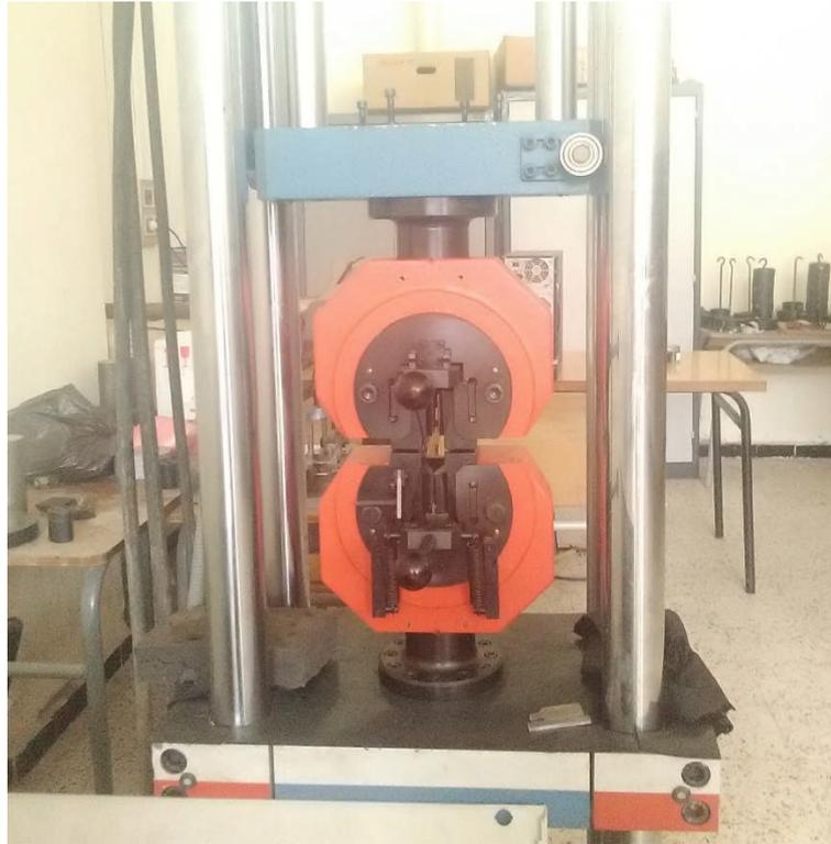
Figure III.16: Machine de traction.
