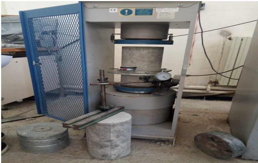
FIGURE 4.7 – Essai de compression uni axial.
