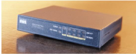
Figure III.15 : Cisco PIX Firewall
