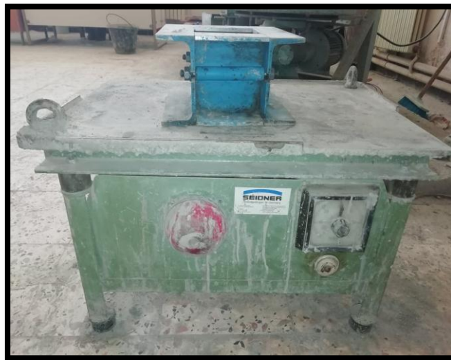
Figure 12: vibration des moules.
