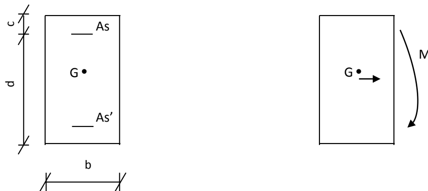
Figure III.3.2: section de balcon.
