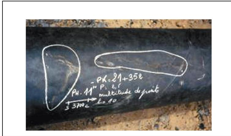
**Figure.II.14a** multitude de points de corrosion [11]
