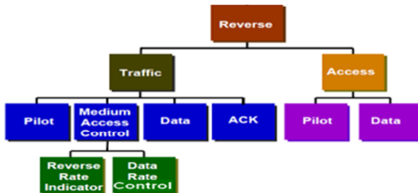
Figure III.8 : Structure du canal montant.
