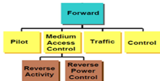
Figure III.5: structure du canal descendant.
