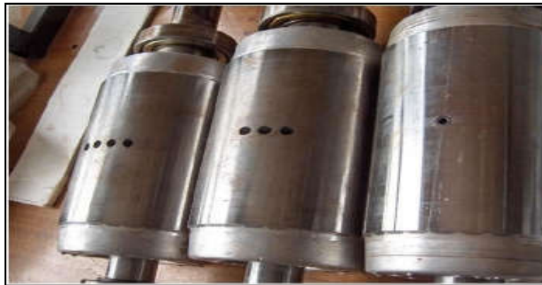
Figure I-12 : Rupture de barres [9]
