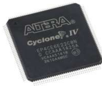
Figure (I.11) : FPGA, Altera, EP4CE6E22C8N, Cyclone IV E, 6272 Cellules, 392 Blocs, EQFP 144.
