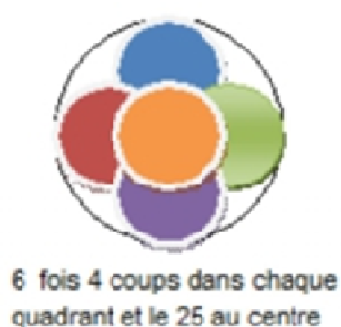
Figure : [VI.6] Compactage des couches.
