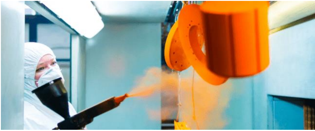
Figure III.17: Méthode de thermolaquage.
