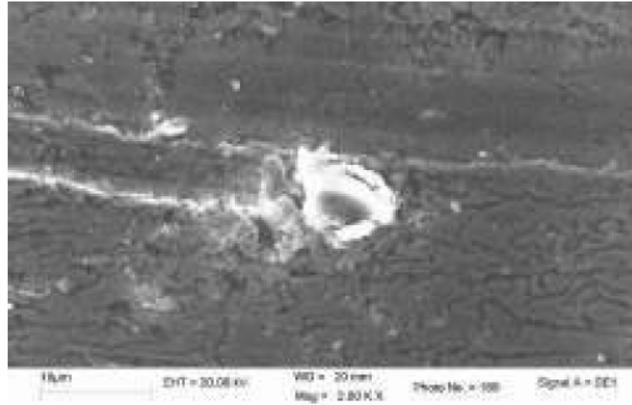
Figure I.5 : usure abrasive [2]
