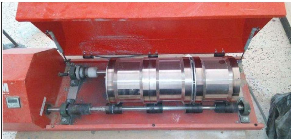
Figure V.1.Appareillage Micro Deval.
