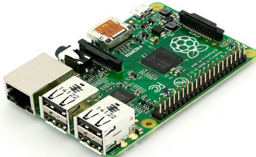
**Figure II.4:** Raspberry PI Model B+. [9]
