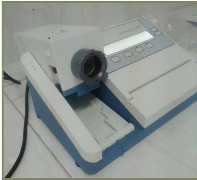
Appareil digital de type Melting point Apparatus, SMP30
