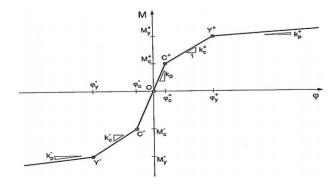
Fig .2 Moment -curvature response of modified TAKEDA model [16].
