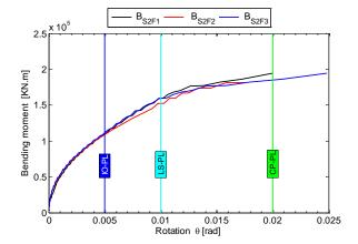
Fig .6 Moment- rotation relations developed in the beams of RC frame (Beams of 2<sup>nd</sup> level).
