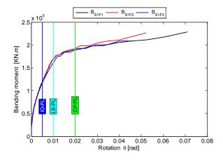
Fig .5 Moment- rotation relations developed in the beams of RC frame (Beams of the 1st level).
