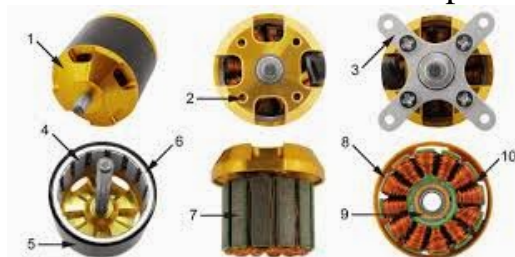
Figure III.7 : moteur Brushless outrunner
