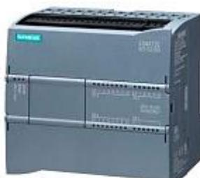
\*\*\*Spare part\*\*\* SIMATIC S7-1200, CPU 1214C, compact CPU, DC/DC/relay, onboard I/O: 14 DI 24 V DC; 10 DO relay 2 A; 2 AI 0-10 V DC, Power supply: AC 20.4-28.8 V DC, Program/data memory 50 KB
