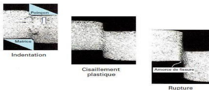
Figure II. 25: Phases de poinçonnage.
