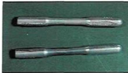
Figure II. 3-b: Epreuves de traction.
