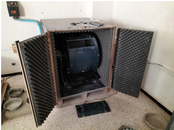
Figure IV.6 : Machine Los Angeles
