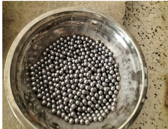
Figure IV.9 : Charge abrasive du Micro-Deval
