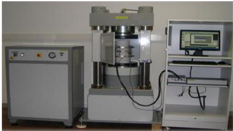
Figure 2.7 : Machine hydraulique HP 3000 KN.
