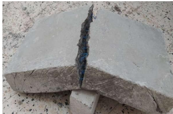
Figure V.13 Mode de rupture de dalles (GPP/PM)
