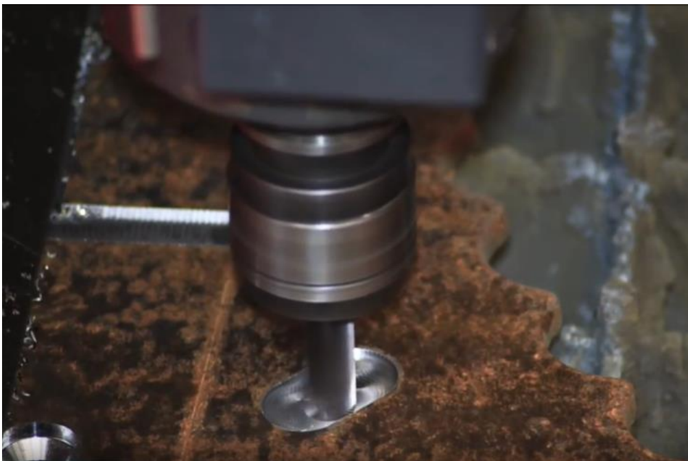
Figure 10 : Surfaçage et rainurage
