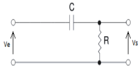
Figure II.6: Filtre passif "passe-bas" Figure II.7: Filtre passif "passe-haut"
