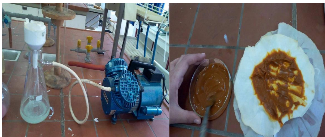
Figure II.2 : Lavage et filtration.
