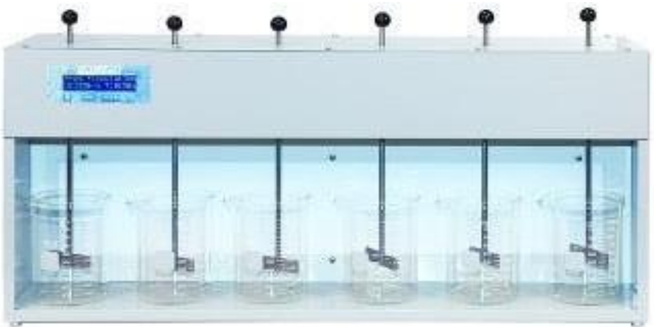
Figure III.3 : Essai de jar-test.
