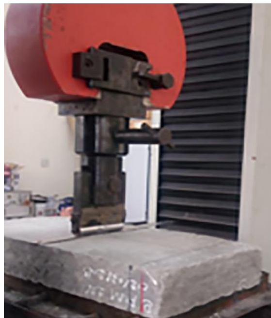
Figure III.12 Dispositif et principe de support à 3-points
