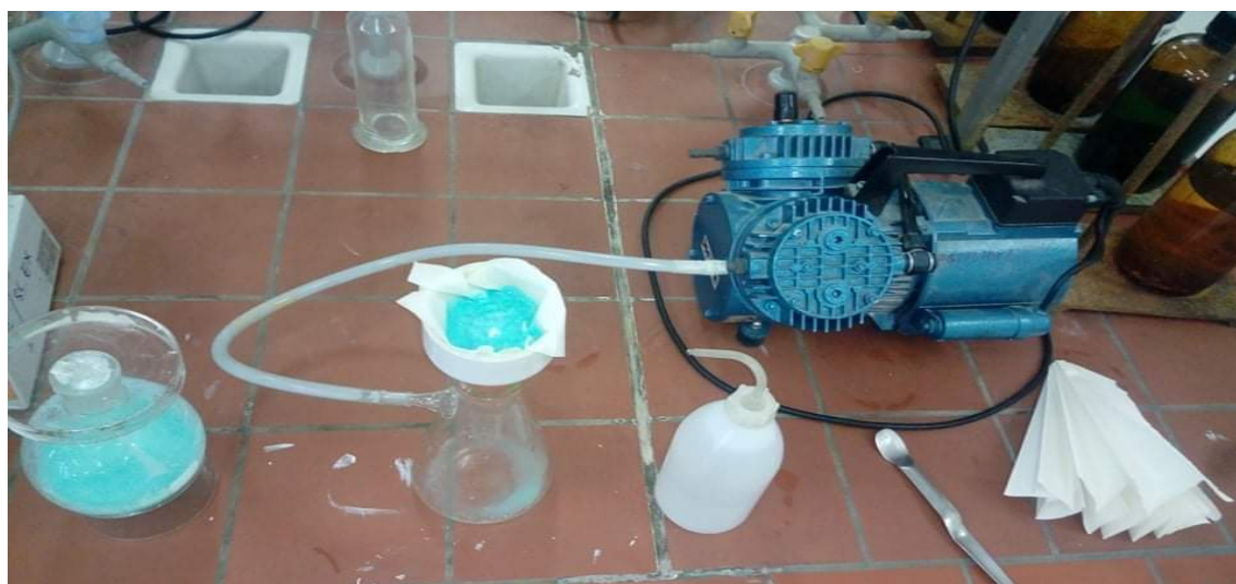
Figure III. 3. Filtration et lavage.
