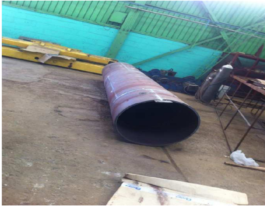
Figure II.6 : tube de foyer lisse de la MYRA4000.
