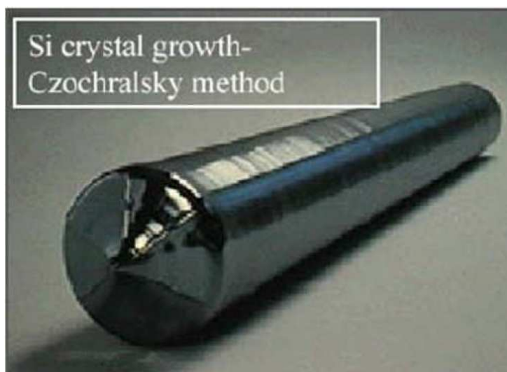
Figure I.23: Le lingot du silicium.
