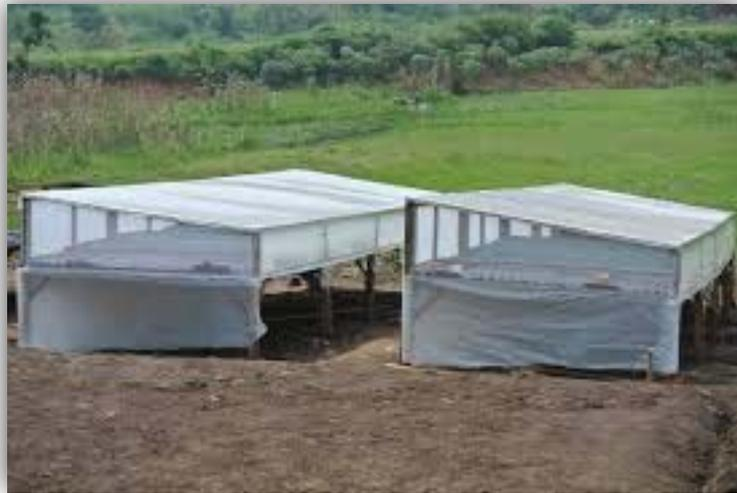
Figure I-15: Séchoir solaire cabane.
