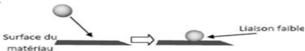
Figure I-5 : Principe de la physisorption.
