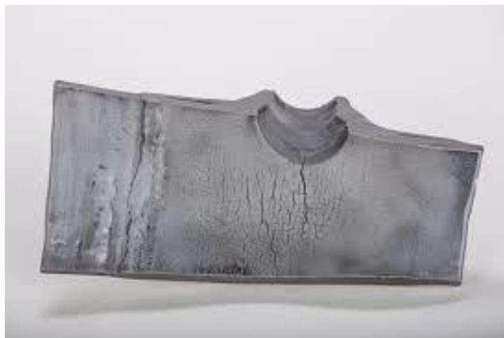
Figure II.5: corrosion sous contrainte
