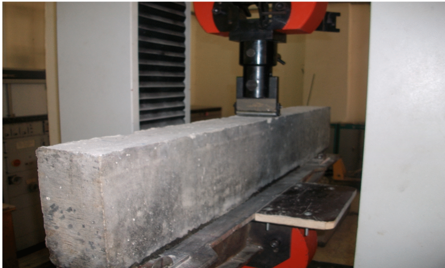
Figure IV. 7 Exemple d'essai flexion 3-points.
