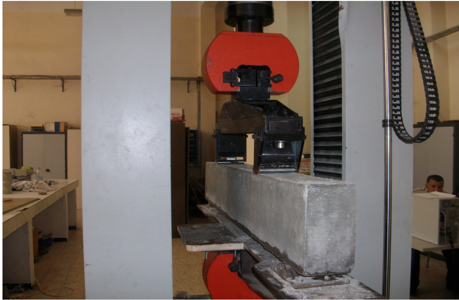
Figure IV. 14 Exemple d'essai flexion 4-points.
