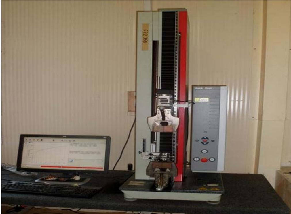
**Figure IV.10 :** Machine de traction type Zwick/Roell Z2.5.
