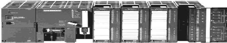
**Figure II.1 :** Automate programmable S7-300 Siemens.
